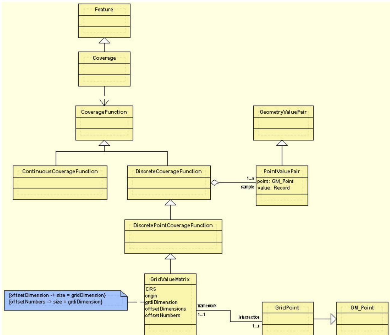
**Figure 6:** Simplified view of the abstract model introduced by ISO 19123
