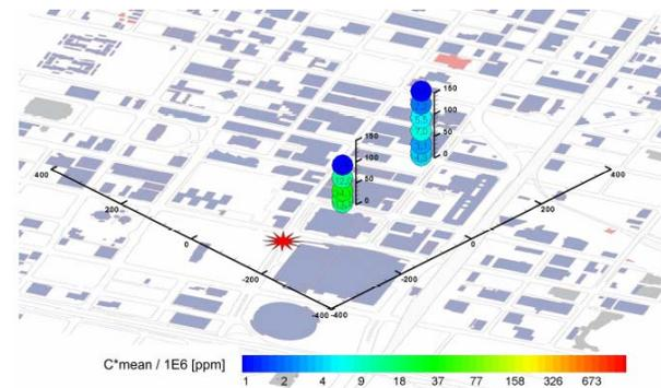
Fig. 7: Vertical profiles of mean concentration for source 1 and wind direction SSW
