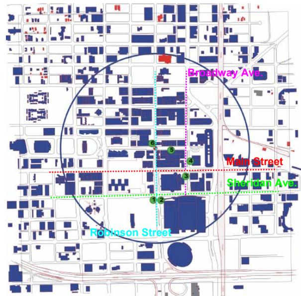
Fig. 1: Map of the Oklahoma City central business district. The circle indicates the area reconstructed in the wind tunnel and the numbers different source locations studied in the wind tunnel.
