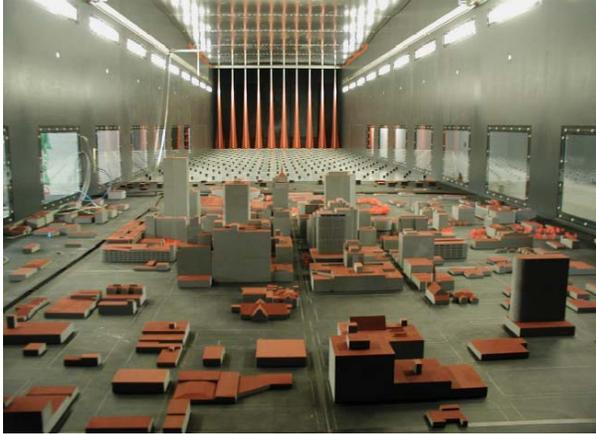
Fig. 2: Model of the Oklahoma City central business district installed in the wind tunnel.
