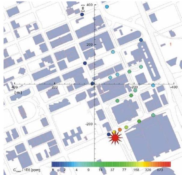
Fig. 6: Mean concentration 3m above ground for source 1 and wind direction SSW
