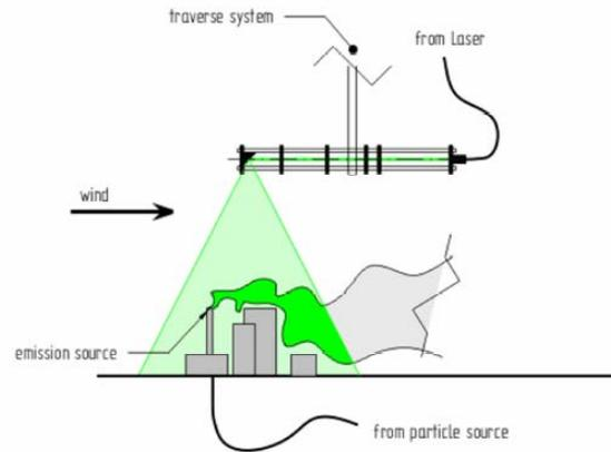
Fig. 3: Schematic view of the laser light-sheet setup.
