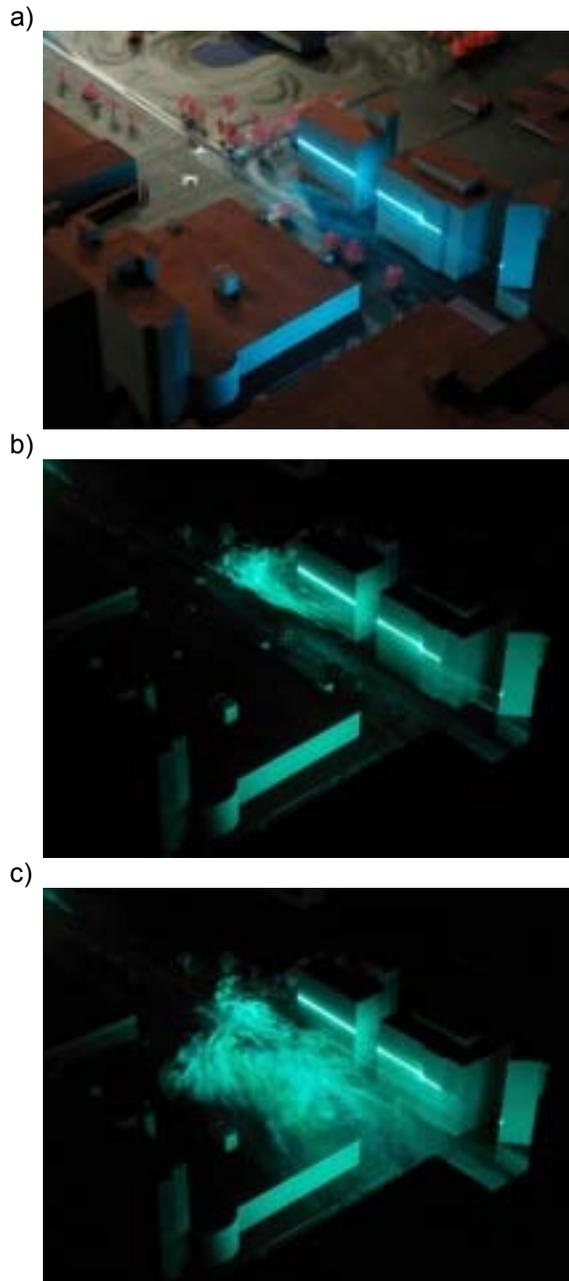
Fig. 4: Laser light-sheet visualization for source 1 and wind direction south. The light sheet is oriented horizontally at about 20m above ground (plot a). The two snapshots (plots b and c) illustrate the instantaneous behavior of the plume.
