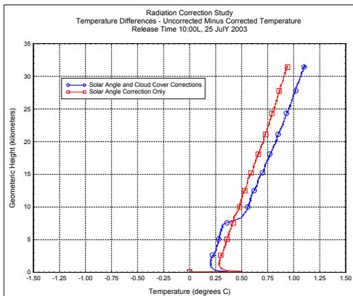
Figure 4. Temperature difference plot for raw minus corrected data sets.
