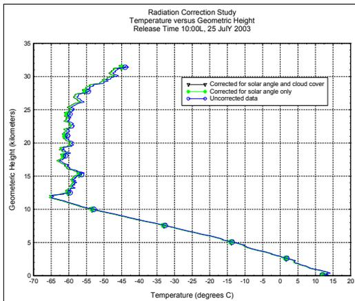
Figure 3. Temperature profiles for the raw and corrected data sets.
