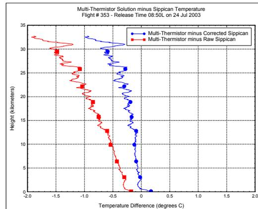
Figure 6. Temperature difference plots multi-thermistor minus Sippican.
