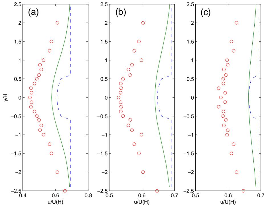
Figure 3: Plot of the streamwise velocity component as a function of the crosswind direction ( $y$ ) near the ground ( $z/H=0.1$ ) as calculated using the original Röckle (1990) model (— — —), the shelter model (—), and the SL94 data (o) at three streamwise locations far downstream of the cube: (a)  $x/H = 4$ , (b)  $x/H=6$ , (c)  $x/H = 8$ .
