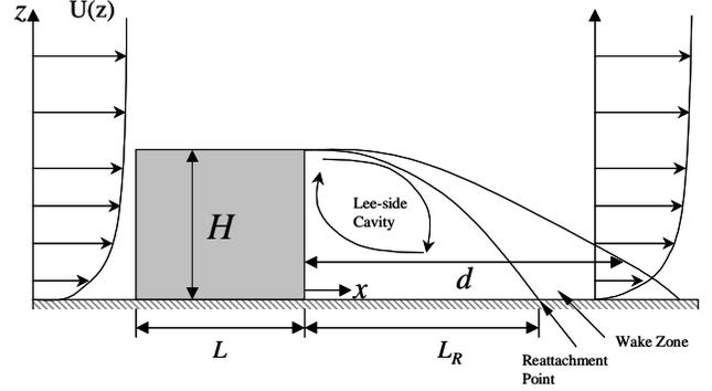
Figure 1: Schematic of flow in the wake of a building.
