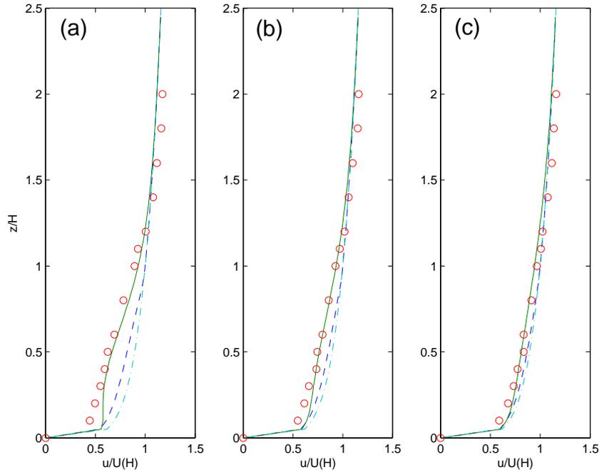
Figure 2: Plot of the streamwise velocity component as calculated using the original Röckle (1990) model ( - - - ), the shelter model ( ——— ), and the SL94 data (○) at three streamwise locations far downstream of the cube: (a)  $x/H = 4$ , (b)  $x/H=6$ , (c)  $x/H = 8$ . Also shown is the upstream boundary layer profile ( - · - · ).
