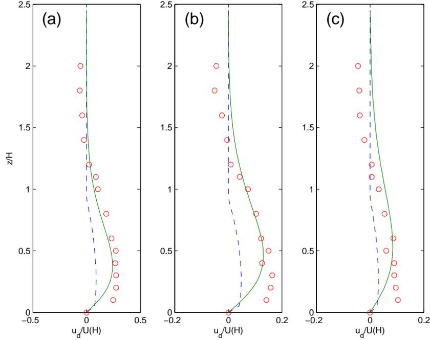
Figure 1: Plot of the streamwise velocity deficit as a function of the wall normal distance ( $z$ ) as calculated using the original Röckle (1990) model (— — —), the shelter model (— — —), and the SL94 data (o) at three streamwise locations far downstream of the cube: (a)  $x/H = 4$ , (b)  $x/H = 6$ , (c)  $x/H = 8$ .
