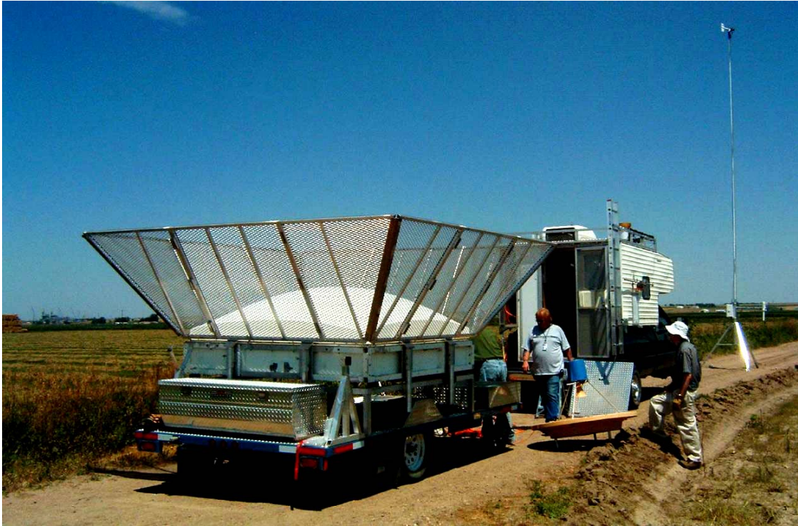
Figure 1: The MISS wind profiler, camper, and instrumented tower deployed on 1 Aug. 2003, southeast of Hudson, Colorado. (photograph © H. Bluestein).
