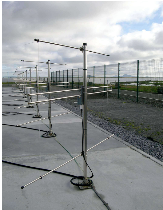
Fig. 2 Pictures of antenna field plus close up of individual Yagi antenna
