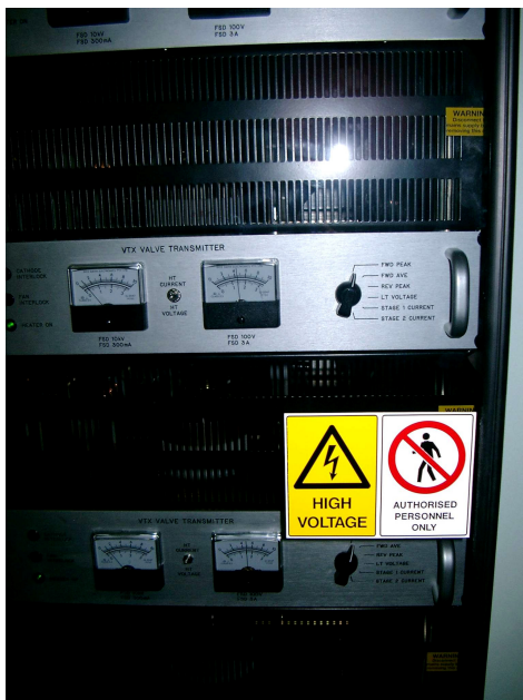
Fig. 3 LHS rack mounted transmitters, RHS two electronics cabinets house the basic hardware
