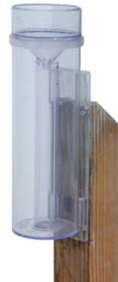
Figure 1. The CoCo RaHS rain gauge is a clear plastic gauge four inches in diameter suitable for use in all seasons and weather conditions. This gauge is able to measure accurately in increments of 0.01” and can hold up to a total of 11 inches of rain without spilling. It is used extensively by the National Weather Service in weather spotter networks.
