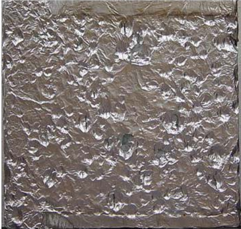
Figure 2. A CoCo RaHS “Hail Pad” showing the clearly visible dents caused by a recent hail storm.
