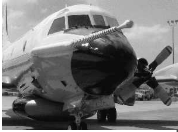
Fig 1: BAT probe mounted on NOAA P3 research aircraft. The probe protrudes roughly 4-5 m in front of the fuselage nose.
