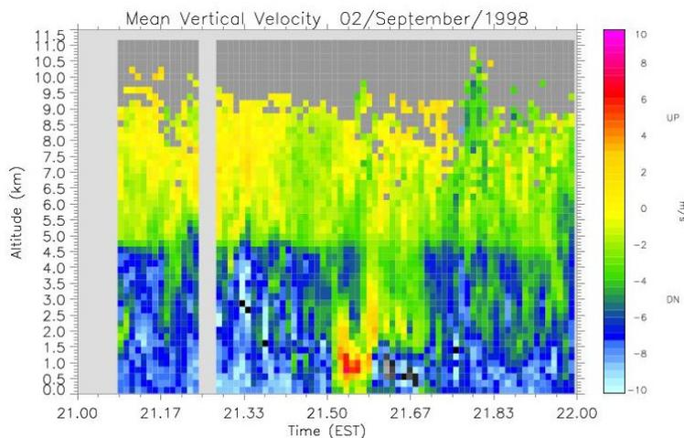
Figure 3. MIPS 915 MHz Doppler Wind Profiler Vertical Velocity
