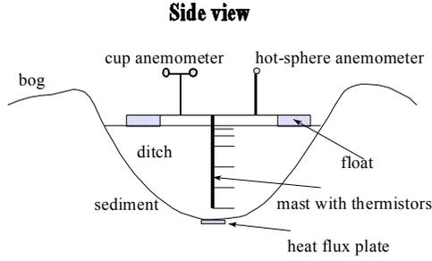
**Figure 1:** Outline experimental set-up.
