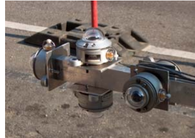
Figure 2. Pyranometers for measuring short-wave radiation from the three-dimensional surroundings of a standing person.
