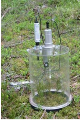
Picture 1 The soil respiration chamber and the measurement setup for the trial measurements conducted at the Hyttiala Forestry Field Station in Hyttiala, Finland
