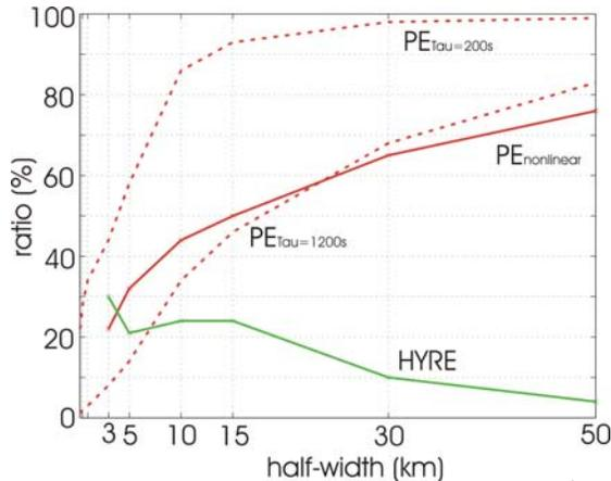
FIGURE 3: Efficiency versus mountain width.  $PE^I$  (broken line) for both  $\tau=200s$  and  $1200s$  is shown. Re-evaporation of hydro-meteors (HYRE) is also indicated.
