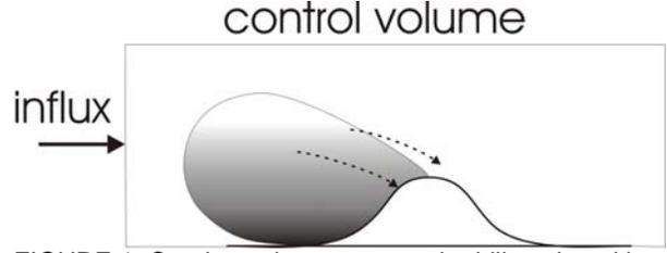
FIGURE 1: Condensation upstream the hill enclosed in a control volume.
