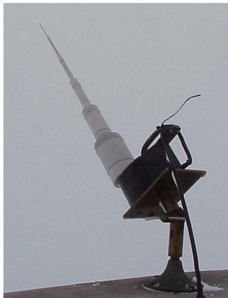
Figure 1. Rotating multicylinder exposed to cloud at MWO.
