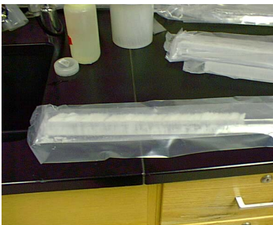
Figure 2. Sample rod with ice in sealed bag for transport from MWO to analysis lab at the University of New Hampshire.
