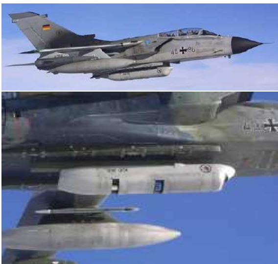
Fig. 5: The center-line pod under the aircraft contained the IR camera.
