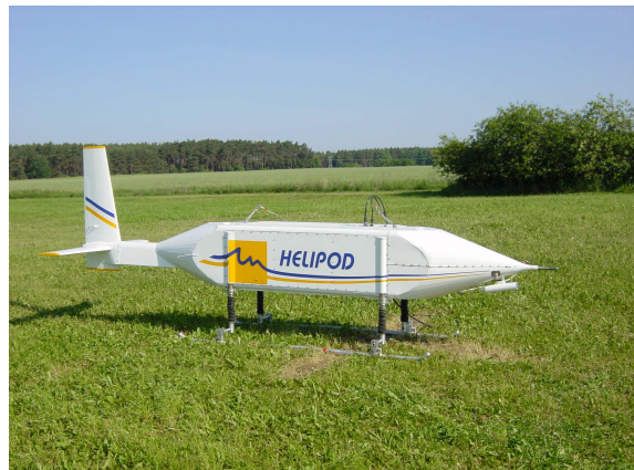
Fig. 3: The helicopter-borne turbulence probe Helipod.
