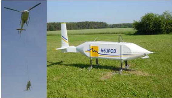
Fig. 2: The helicopter-borne turbulence probe Helipod.
