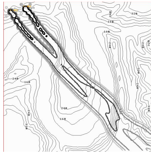
Figure 13. Two adjacent plumes being dispersed, in a northwesterly flow field, into the valley, combining and then collecting at the southeast wall
