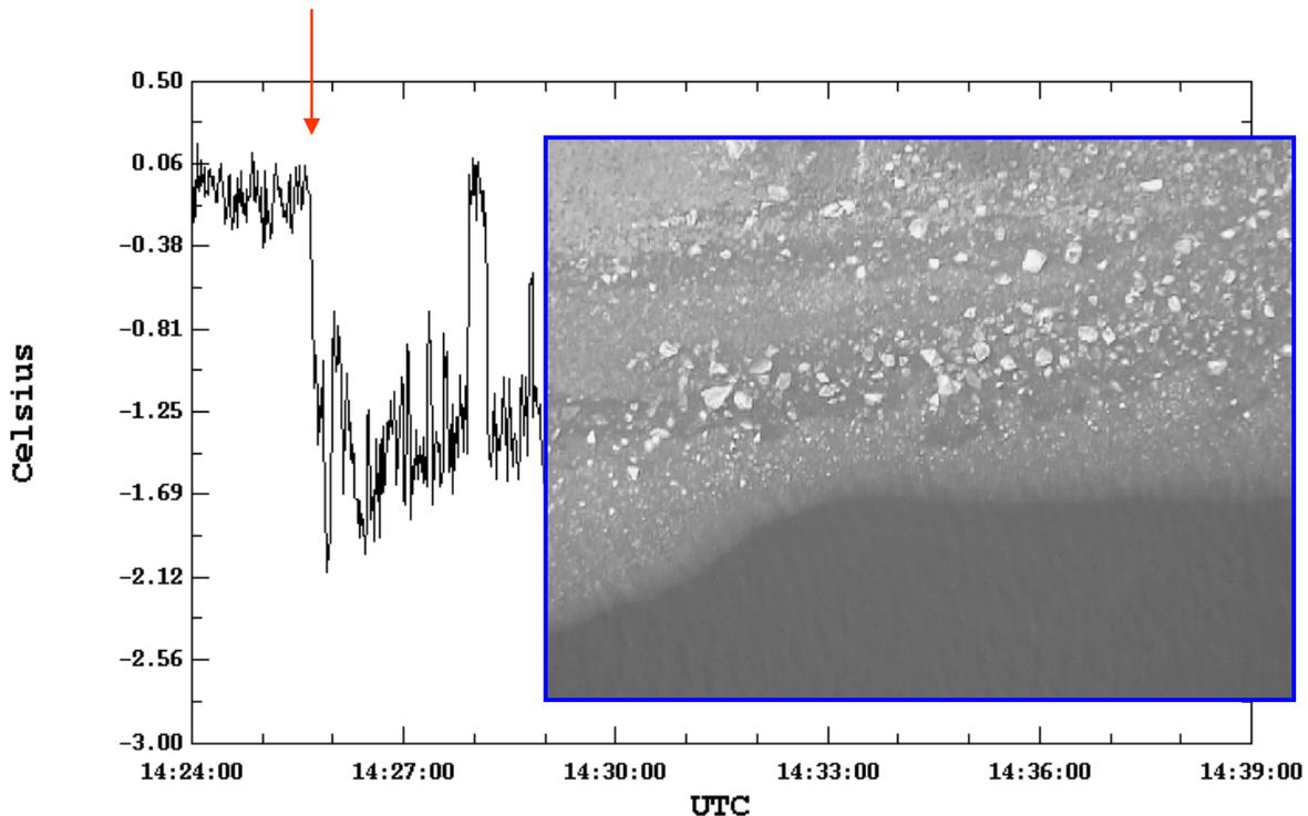
Figure 3. Example of changes in Heimann radiometric temperature when the aircraft flew over a water-ice boundary. The plot is of Heimann radiometric temperature as a function of time on 26 February 2004. The red arrow shows the time of the inset video image. In the video image, the aircraft is flying from bottom to top.
