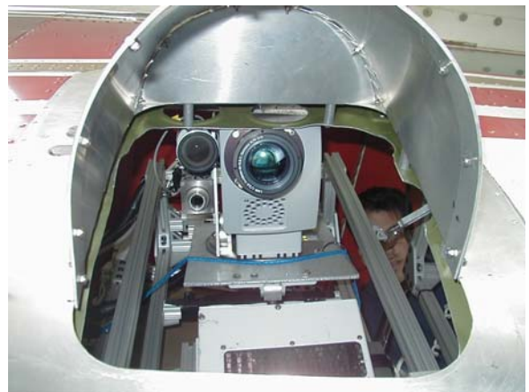
Figure 1. (Top) Cessna Skymaster flown during CBLAST-LOW 2002/2003 based in Chatham, MA. (Bottom) Close-up of the downward-looking IR imager, collocated video camera, and collocated, narrow FOV IR radiometer.
