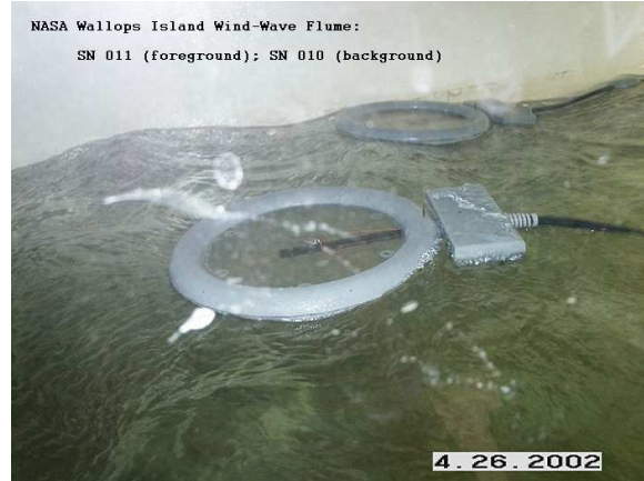
Figure 1: Multi-sensor floats; Greenland Sea design during testing in NASA wind-wave flume.
