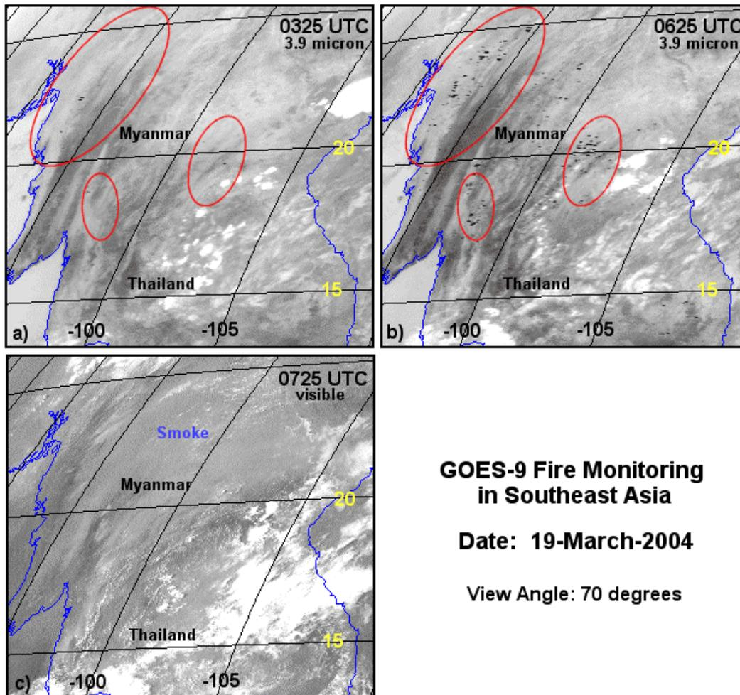
Figure 3. Fires observed in GOES-9 visible and 3.9  $\mu\text{m}$  imagery in southeast Asia on 19 March 2004. The dark hot spots in the 3.9  $\mu\text{m}$  imagery are fire pixels.
