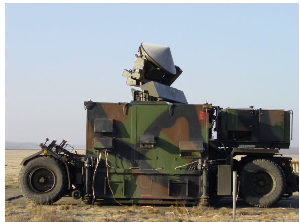
Figure 1: Flycatcher radar with pencil beam used to track single targets.
