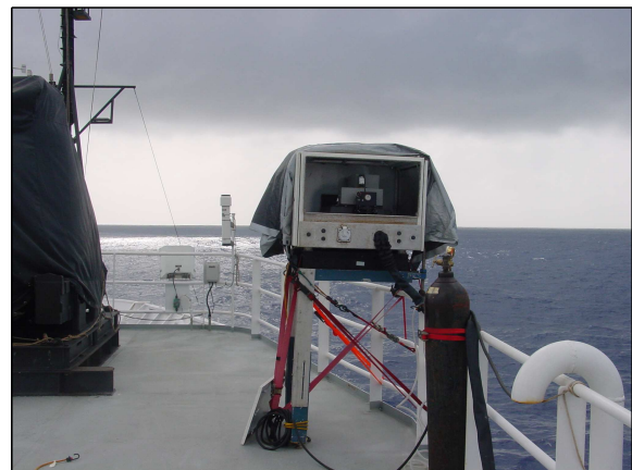
Figure 4: The UM/RSMAS Marine Atmospheric Emitted Radiance Interferometer (M-AERI) onboard the Ronald H. Brown during AEROSE Leg 2 operations in March 2004.
