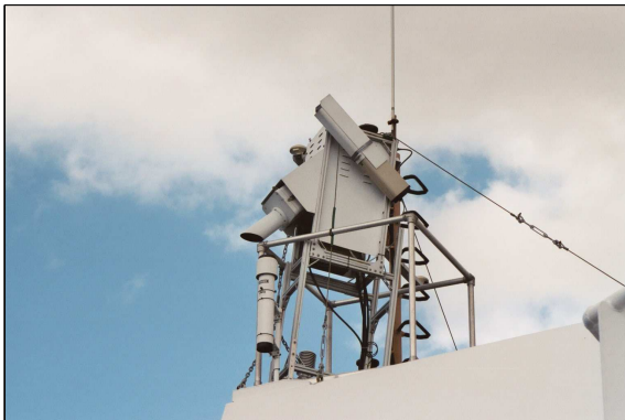
Figure 5: The UW/APL Calibrated Infrared In situ Measurement System (CIRIMS) onboard the Ronald H. Brown during AEROSE.
