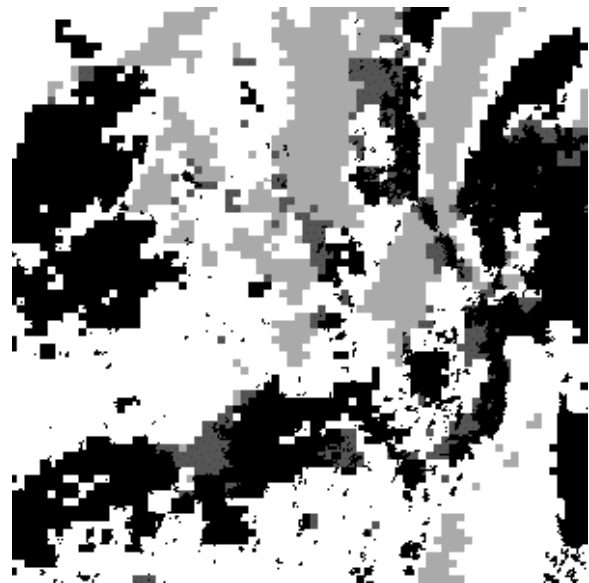
Figure 4. Results of multispectral image classification for 2020 UTC on 9 April 2002 over study region (same geographic area as Figure 3), showing scaled images of pixel types [black=land, dark gray = snow, light gray=ice cloud, white = water cloud].
