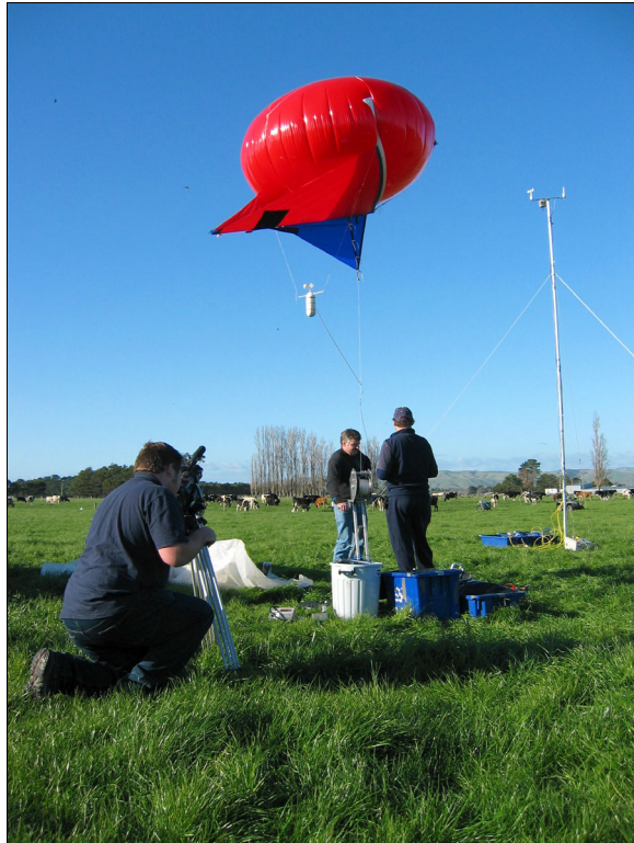
Figure 1: Helikite being raised with suspended radiosonde and sampling tubes at several heights.
