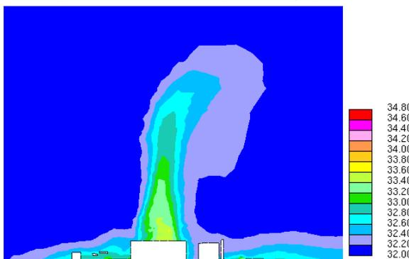
Fig.17 Vertical temperature distribution (°C)
