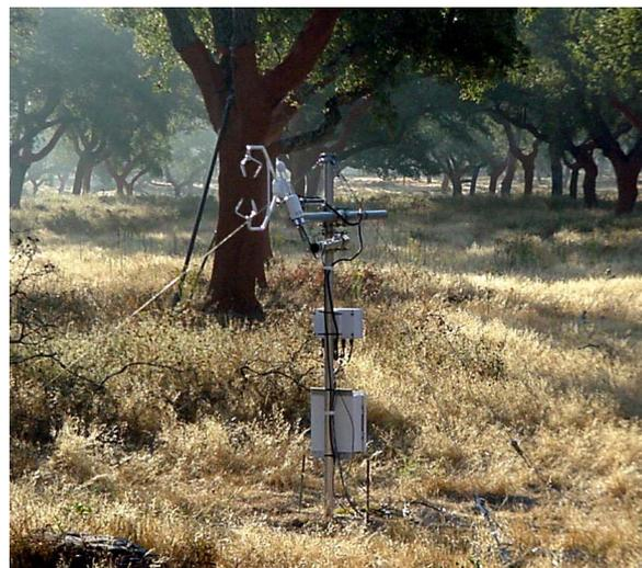
**Fig. 2:** One of the eight (identical) 1.8 m masts in the trunk space equipped with a Campbell Scientific CSI CSAT 3. The photo shows position C5.
