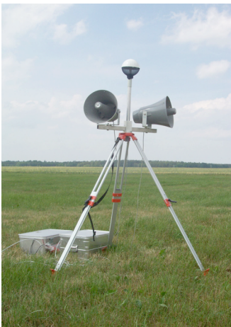
Figure 4. Example of combined sound source and receiver at a tripod. The measuring microphone (with a windscreen) is mounted at a tube above the twin speakers (pressure chambers).
