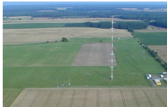
Fig. 1: View of the experimental area at the boundary layer research site near the Lindenberg Meteorological Observatory of the DWD. The 99m meteorological tower (foreground), the grassland and the ploughed field are visible.
