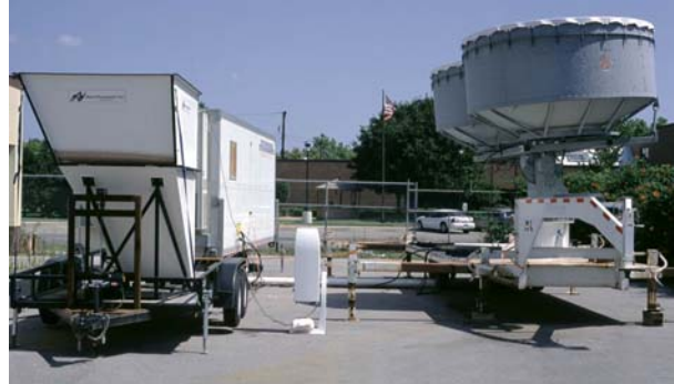
Figure 1 – The DPG FM-CW Radar located in Oklahoma City for the Joint Urban 2003 Urban Dispersion Experiment. Also shown are the DPG SODAR (left, in front of the electronics trailer) and the Lawrence Livermore National Laboratory ceilometer.
