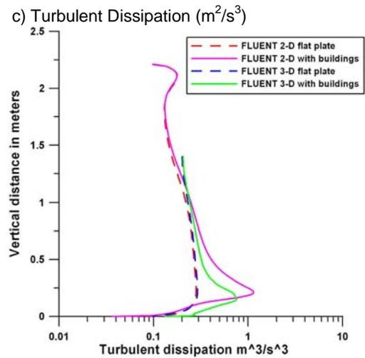
Figure 7. Profiles within the first building canyon.
