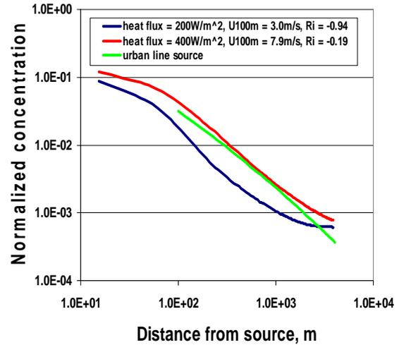
Figure 3. Comparison of normalized concentrations ( $Cu/q$ ,  $m^{-2}$ ) with urban P-G line source.
