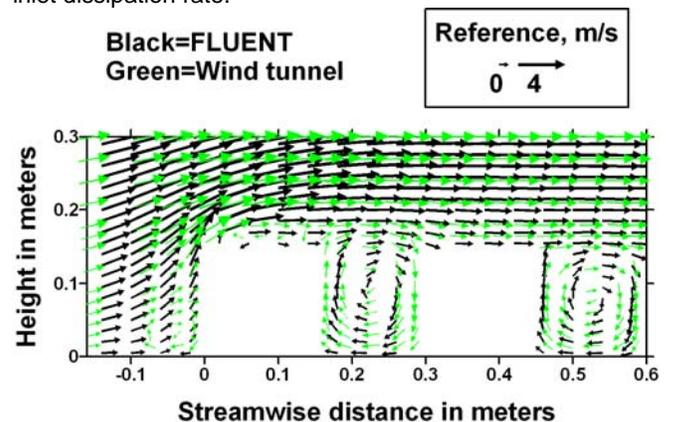
Figure 5. Velocity near two-dimensional buildings.
