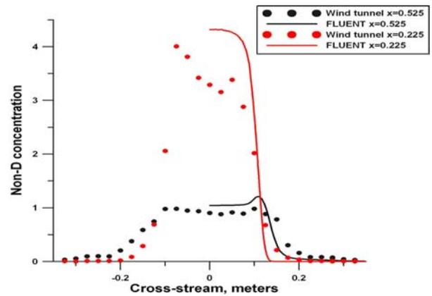
Figure 9. Cross-stream concentration profiles with 1<sup>st</sup> building canyon ( $x=0.225$ ) and 2<sup>nd</sup> building canyon ( $x=0.525$ ).
