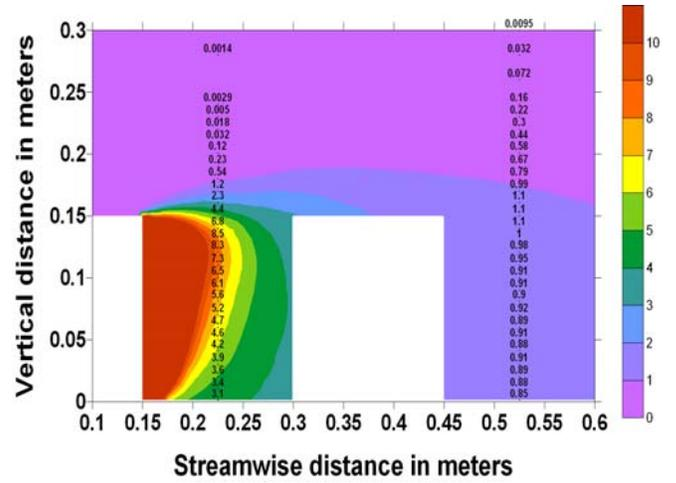
Figure 8. Concentrations within 3-D building canyons at  $y=0$  (CFD color contour, Wind tunnel data numbers).
