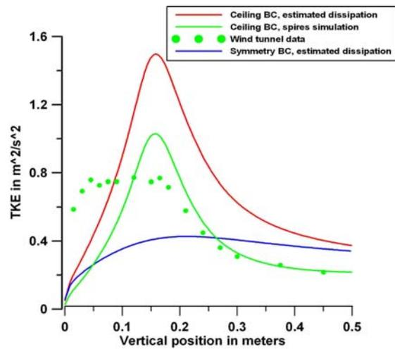
Figure 10. Turbulent kinetic energy in front of leading 2-D building face ( $x=-0.038$  m,  $y=0$ ).
