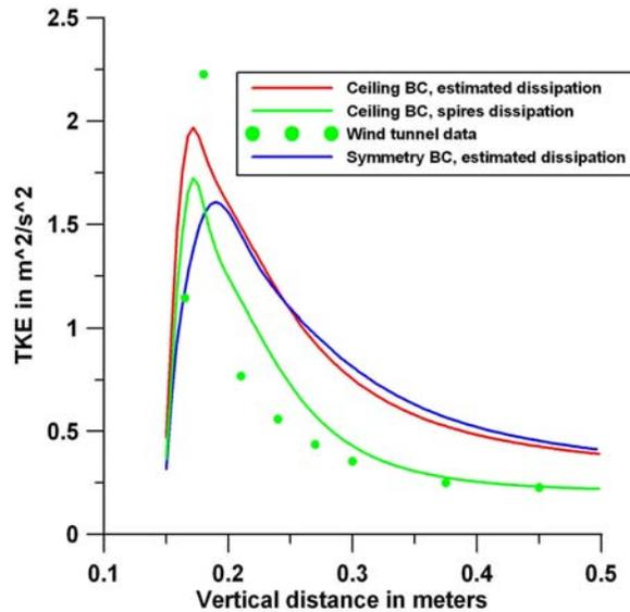
Figure 11. Turbulent kinetic energy on leading 2-D building roof edge ( $x=0.045$  m,  $y=0$ ).
