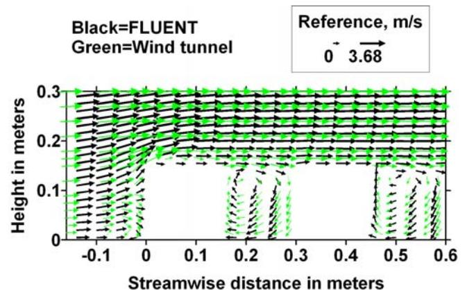
Figure 6. Velocity near three-dimensional buildings.
