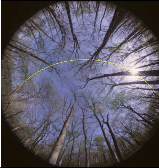
Figure 2 – Hemispherical view of the canopy on April 29, 2004. The calculated path of the solar disk is indicated in yellow.
