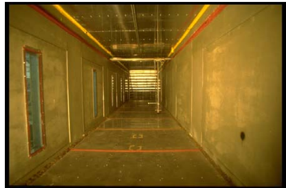
Figure 3. Interior of the UniKa thermally stratified wind tunnel. Winds in the insulated walls of the tunnel are used for laser Doppler flow measurements.
