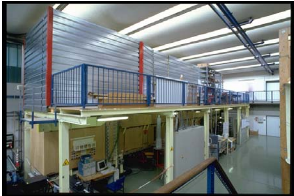
Figure 2. General view of the UniKa thermally stratified wind tunnel with insulated return section (upper part).
