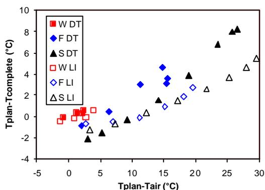
Figure 5. Composite plot of plan-complete surface temperature difference versus plan-air temperature for seasons (W=winter, F=fall, S=summer) and the two study areas (LI and DT).
