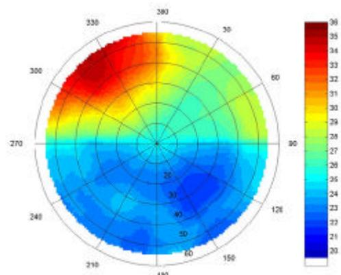
Figure 2. Polar plot of urban thermal anisotropy over the downtown area of Vancouver BC. August 16, 1992 for a 12° FOV airborne sensor (ht 525 m) solar Z=40°, AZ=145°. The colour scale is in °C. The primary street pattern of the area has azimuths of 45° and 135°.
