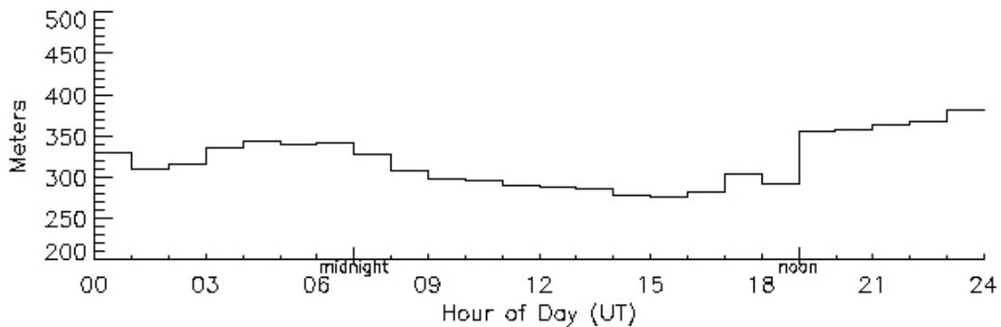
Figure 2. Diurnal variation of the altitude top of the surface reflectivity layer averaged over 11 clear days, 4 – 24 Oct 2000.
