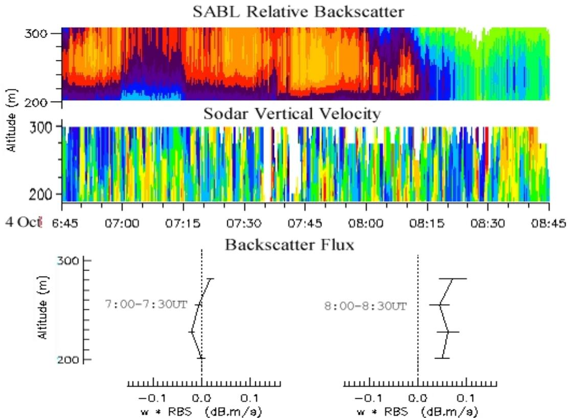
Figure 4. SABL and sodar. The top panel shows lidar backscatter (red/orange is stronger backscatter) and the middle panel shows corresponding sodar vertical velocity (orange/red is upwards, green/blue is down). The lower panel shows profiles of backscatter flux (the product of backscatter and vertical velocity perturbations) averaged over the time periods indicated.
