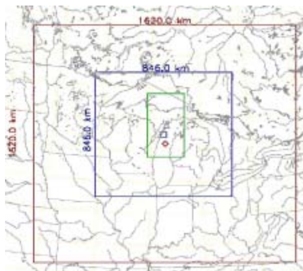
Figure 3: ARPS simulation domains. (1) Regional [91x91 grid, 18km horizontal spacing], (2) Subregional [142x142 grid, 6km spacing], and (3) ng].
