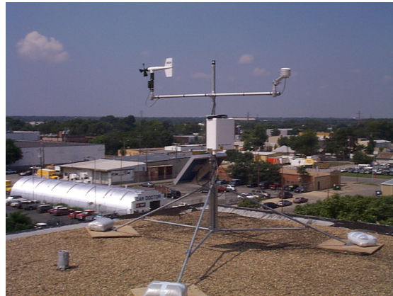
Figure 1. Photo of a tripod-mounted PWIDS located on a roof in Oklahoma City.
