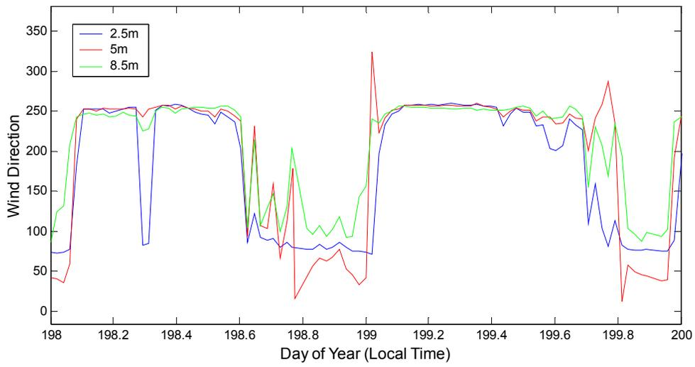
Figure 3. Time series of wind direction measured in street canyon.
