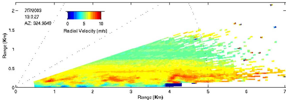
Figure 5. RHI (azimuth fixed at 324.96°, elevation changes from 0 to 20°) LiDAR scan towards CBD
