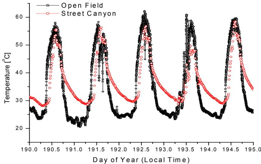
Figure 1. Surface temperatures measured in Park Avenue street canyon and in an open grassy field.
