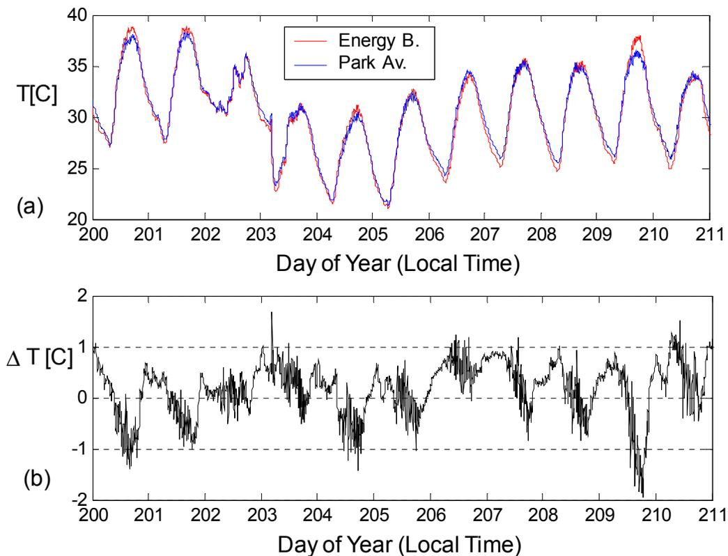
Figure 2. (a) Air temperatures at 8.5m measured in the street canyon and in an open grassy field
