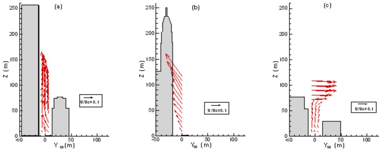
Figure 5. Velocity vectors on the downwind side of tall buildings (shown in silhouette on the left side of each figure. a) Chase Manhattan building (Federal Reserve building on right), b) Woolworth building, c) unknown building approximately 300m northeast of WTC site.
