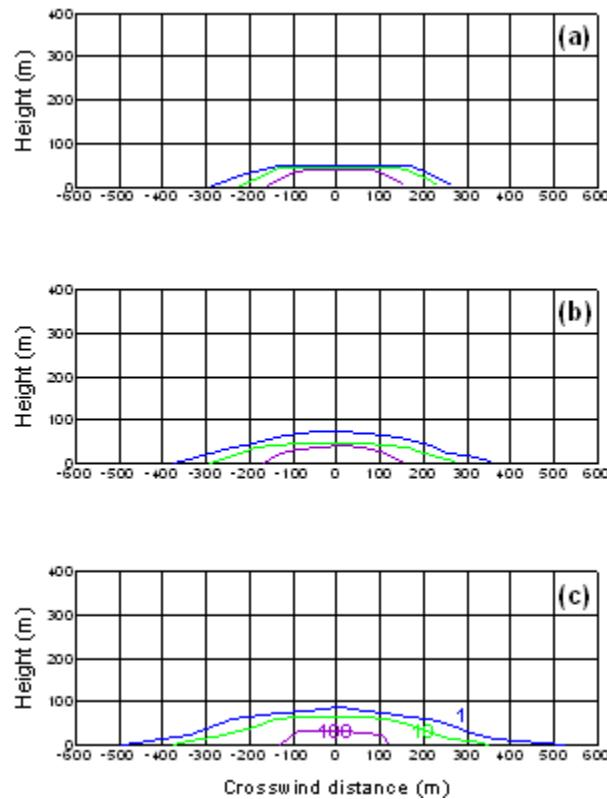
Figure 7. Gaussian plume model results using AERMOD. Plume cross sections at downwind distances of: a) 300m, b) 600m, and c) 1200m. View looking upstream.
