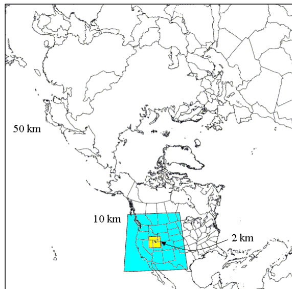
Figure 2. Domain for 50-km hemispheric ARPS simulations with sample locations and coverage of 10-km (blue-shaded) and 2-km (yellow shaded) grids to be used for mesoscale observing system simulation experiments.
