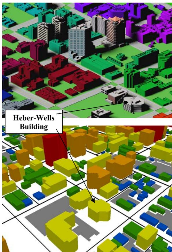
**Figure 3.** Comparison between a high-detail building dataset (top) and a coarse dataset (bottom) for small section of downtown Salt Lake City. The Heber-Wells Building is identified in both for frame of reference.
