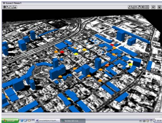
Fig. 12 – A 3D View of the neighbourhood studied with the spatial distribution of the average consumption in graduated colour.
