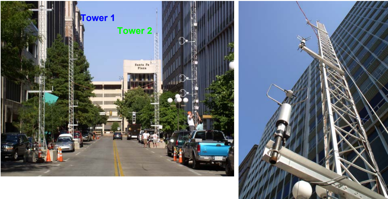
Fig. 2: Photos of the two towers mounted in Park Avenue (left) and close view of the RM Young sonic anemometers installed on tower 2 (right).
