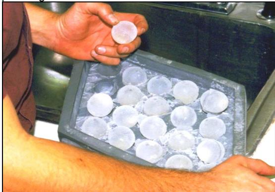
**Figure 2.** Ice ball mold.
