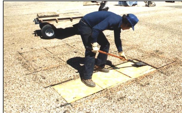
**Figure 1.** Roof samples being removed for impact testing in the laboratory from a 14-year-old roof in Dallas, Texas.
