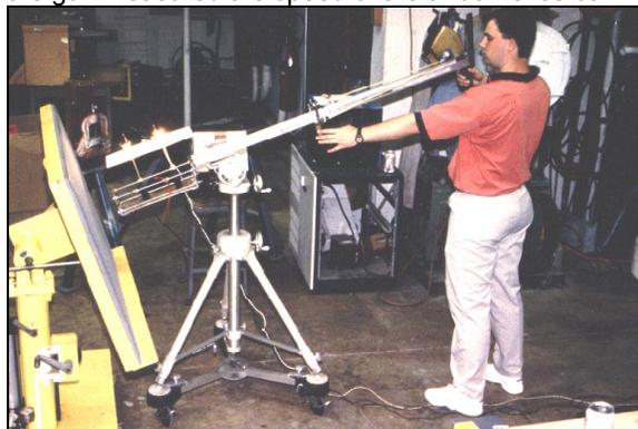
**Figure 3.** Mechanical launcher used to propel smaller ice balls.
