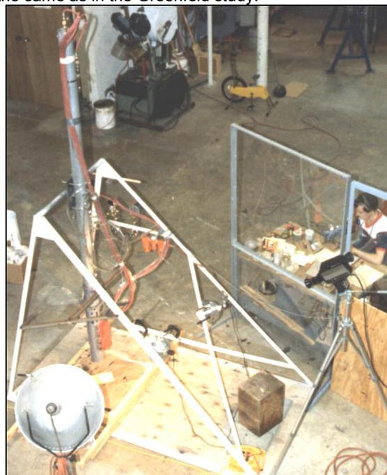
**Figure 4.** Pneumatic air launcher used to propel larger ice balls.
