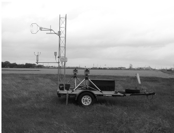
Fig. 1. Mobile measuring unit for calculating CH 4 and NH 3 fluxes from whole farm systems.
