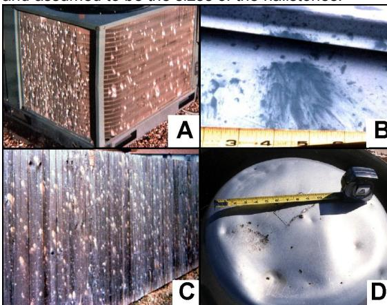
**Figure 7.** Various indirect indicators of hail size and direction: A) dented fins on an air conditioner, B) spatter mark on metal, C) scuff marks on wooden fences, and D) dents in aluminum vent caps.
