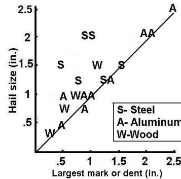
**Figure 9.** Comparison between the largest hailstones with the largest marks or dents on steel (S), aluminum (A), and wood (W) items at 19 locations.
