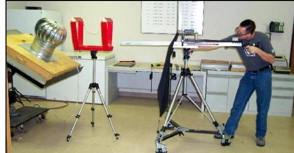
**Figure 11.** Ice ball launcher (IBL-7) utilized to impact various metal items. A chronograph was positioned between the launcher and item to be impacted in order to obtain the velocities of the ice balls.
