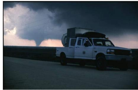
**Figure 1.** The U. Mass. radar collecting data in the Stockton, Kansas tornado on 15 May 1999. View to the northwest. Photograph © H. Bluestein.
