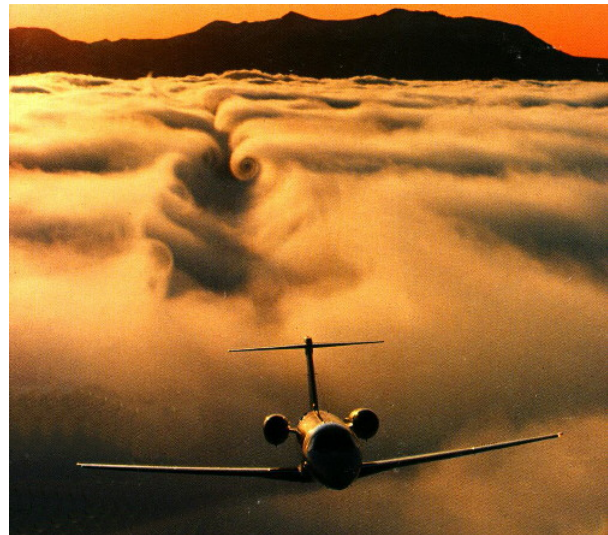
Figure 1: In this photograph, a Cessna Citation VI is flying immediately above a fog bank at approximately 313 km/h or 170 knots (B. Budzowski, Director of Flight Operations, Cessna Aircraft Company, private communication, 1993). Aircraft weight was approximately 8400 kg. As the trailing vortices descended over the fog layer due to the downwash, the flow field in the wake was made visible by the distortion of the fog layer. The aircraft is seen initiating a gentle climb after a level flight, leaving a portion of the fog layer yet unaffected. Photo courtesy of Cessna Aircraft Company. (Higuchi, 1993).
