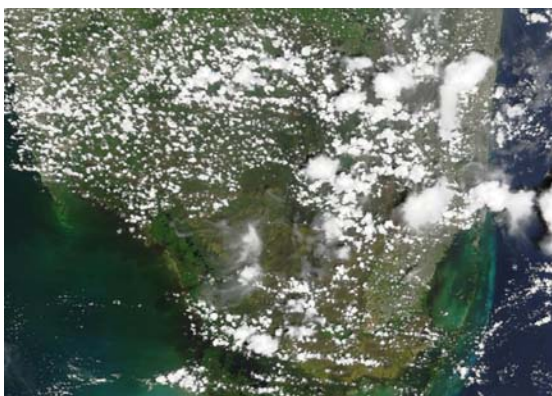
Figure 3. In this hypothetical example, routine 5 minute interval ABI imagery is used to identify a cloud clear region over south Florida which had been cloud covered during the overpass of polar orbiting ocean color satellites. Thus directing the HES VNIR to make its 300 meter resolution measurements.
