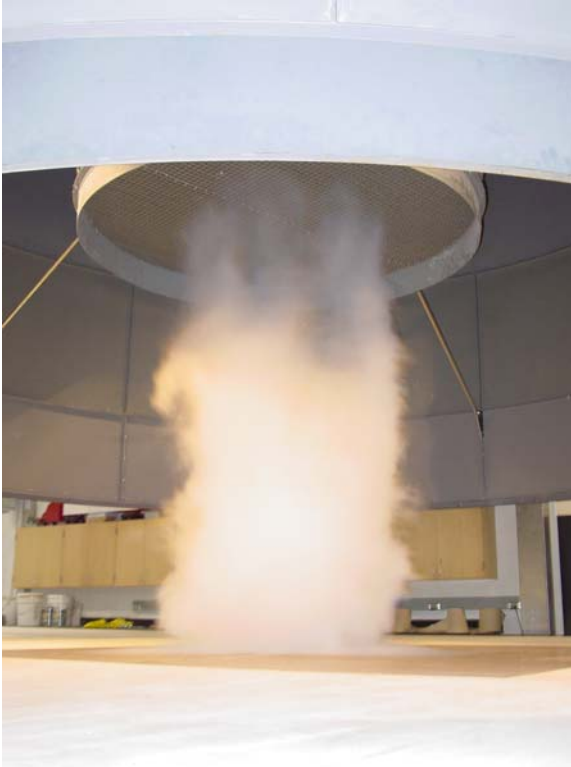
Figure 1: Tornado simulator with vortex highlighted through the use of dry ice.
